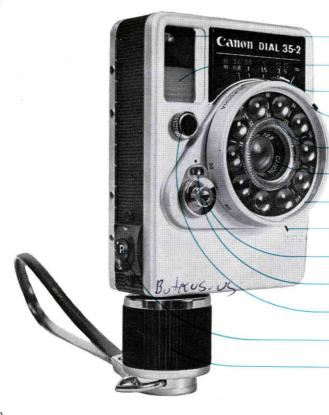
Viewfinder window Illuminating window Focusing lever Film sensitivity index Film sensitivity adjusting lenses on a dial Lens Film sensitivity scale Shutter speed index Shutter release button Exposure counter EE-Flash change button Film rewinding button (R) Spring motor winding grip
